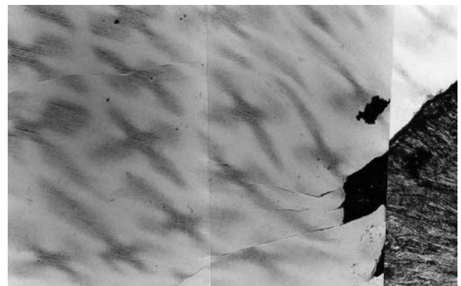
Fig. 10—Micrographs of shear bands formed by deformation without transformation: deformation at 300 K (gray × markings are the product of compositional fluctuations).
